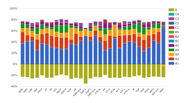
An analysis of the results (environmental impact) has been carried out for the 'generic' product of this LCA and the four variants (colored top layer, each have a share of 25% in the recipe). The result (-9%/+14%) of all individual environmental effects of the individual products are within the margin stated by the NMD (max. +/-20%) for set 1 (EN15808:A1 + 4 additional indicators) when compared to the results of the 'generic' product.
